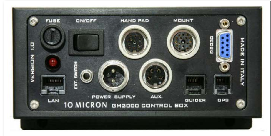
The connections of the control box
